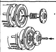
h) Lubricate impeller hub. 3% detergent solution . . . slip new bellows and spring onto impeller hub. Be sure bellows slides freely on impeller hub.
